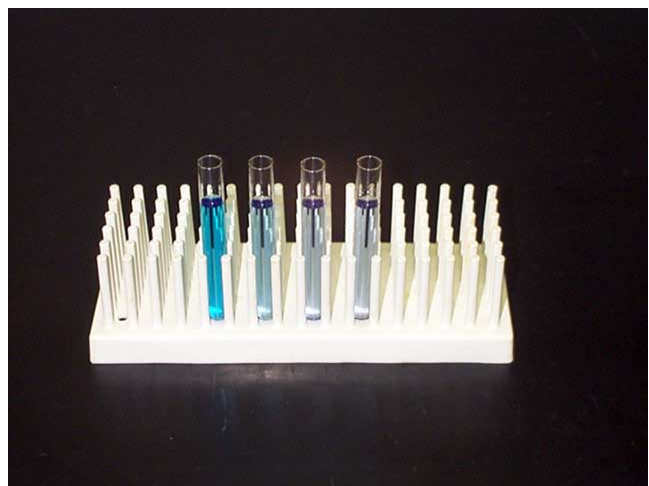
Figure 3. Solutions of \text{Co}^{2+} (21 mM) in 6 M HCl with added (from left to right) LiCl, \text{NH}_4\text{Cl} , NaCl, and KCl.
