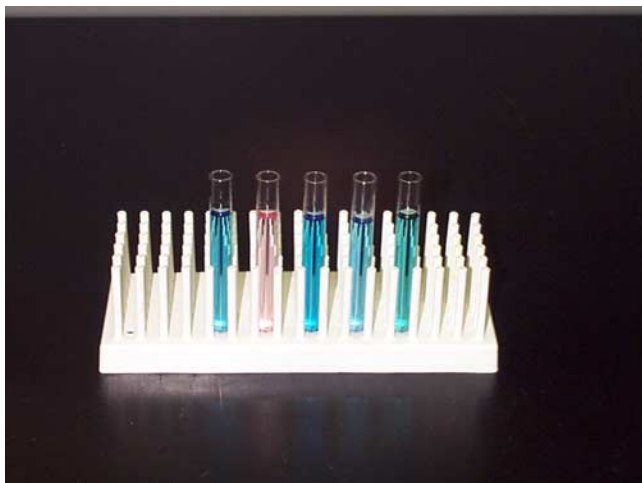
Figure 5. Solutions of \text{Co}^{2+} (21 mM) in 6 M HCl with added (from left to right) \text{H}_2\text{SO}_4 , \text{Na}_2\text{SO}_4 , \text{CaCl}_2 , \text{CaCl}_2 \cdot 6\text{H}_2\text{O} , and \text{MgSO}_4 .
